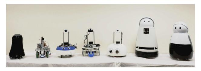
First, Kuri had a custom-built, cost-efficient depth sensor that enabled her to use SLAM (Simultaneous Localization And Mapping) to map customers' homes, even with kids and pets underfoot. It also enabled her to localize within those maps, and navigate independently.
